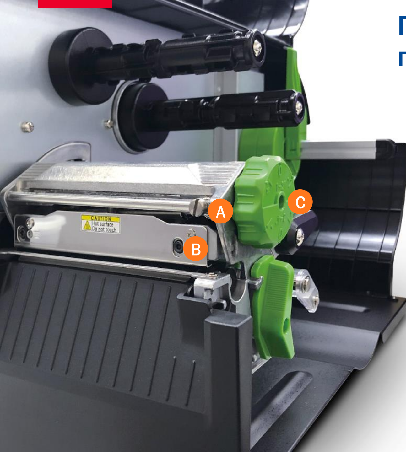
A. Ribbon tension adjustment B. Heat line adjustment
